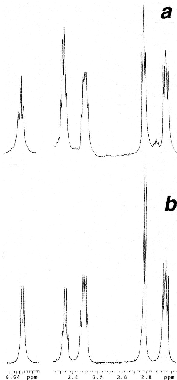
Figure 1. Partial ^1\text{H} NMR spectra of 1a (a) and 1b (b), \text{CDCl}_3 , 23 °C.
